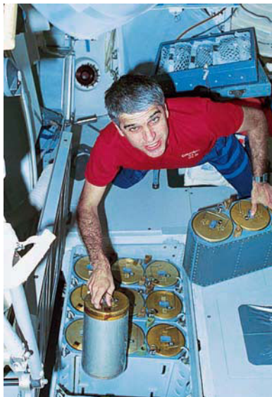
Astronaut Sidney M. Gutierrez changes the lithium hydroxide canisters on space shuttle Columbia. The lithium hydroxide is used to purge carbon dioxide from the air in the shuttle's cabin.
